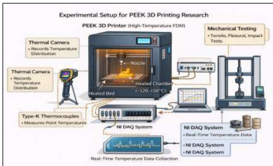
Fig 9 Experimental Setup for Temperature Monitoring, Data Acquisition, and Mechanical
