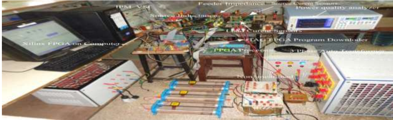
Fig. 3. Experimental prototype of the FPGA-based DSTATCOM.
