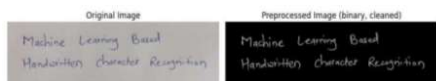
Figure 2. Original photographed handwriting sample (left) and the corresponding preprocessed, binarized image (right).
