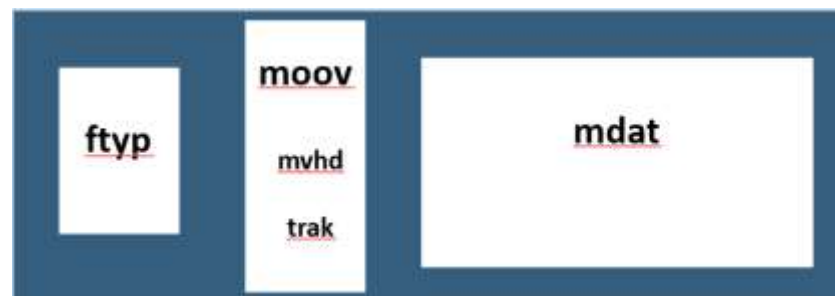
Figure 3: Demonstration of the basic structure of M4A digital audio file
