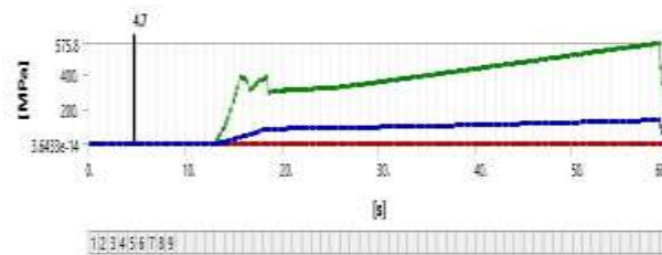
Fig. 19. Equivalent stress (triangular drawbead).
