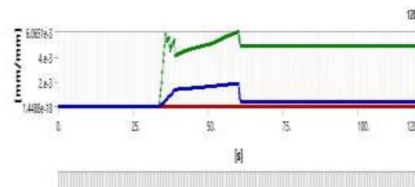
Fig. 12. Elastic strain (square drawbead).
