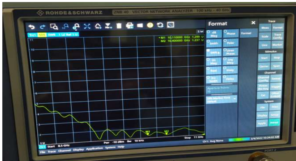
Fig. 11. Practical measured VSWR response after tuning.
