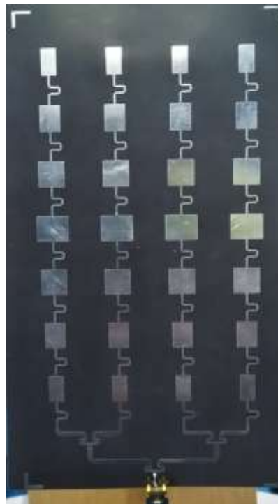
Fig. 3. Fabricated 4 \times 7 microstrip patch array on the Rogers 5880 laminate.
