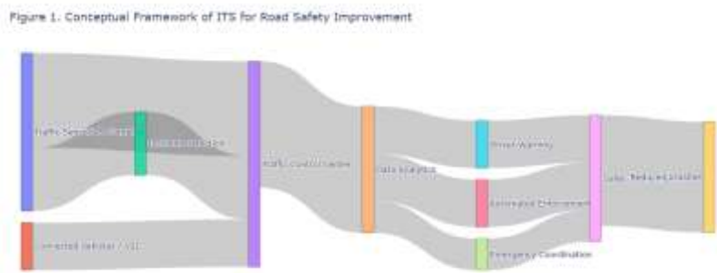
Fig. 1. Conceptual framework of ITS for road-safety improvement, linking sensing and detection (sensors, cameras, connected vehicles), data processing and traffic-control centres, driver warning and enforcement, and emergency coordination to measurable road-safety outcomes.
